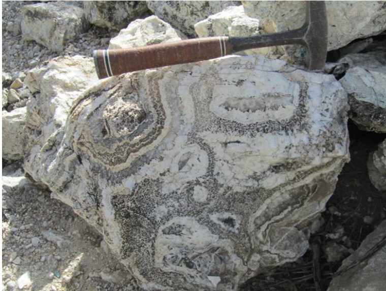
Figure 3. Photo of vein breccia showing well developed crustiform and colloform textures, revealing a complex epithermal history likely due to boiling fluids; Cherokee mine dump
